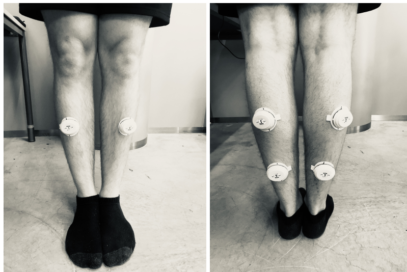
Figure 3.8: EMG sensors' placement
