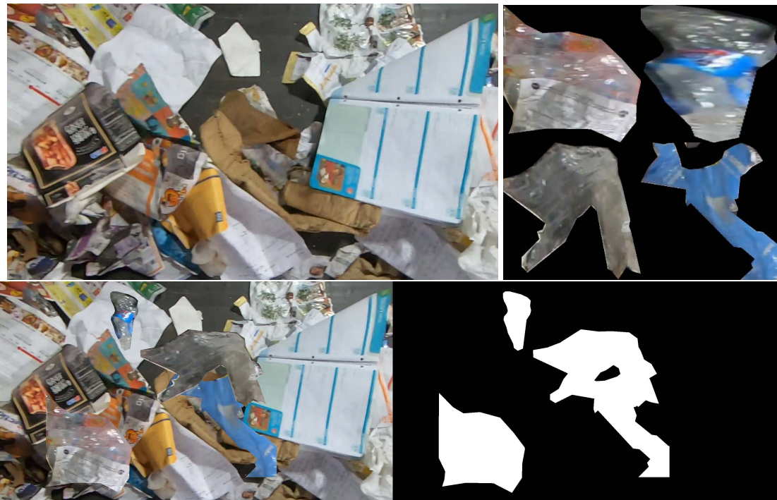
Figure 3.4: On the top left, an example of negative image (background). On the top right, an example of patches retrieved from the ZeroWaste dataset (foreground). On the bottom, the result obtained after copy & paste, with the relative segmentation mask.
