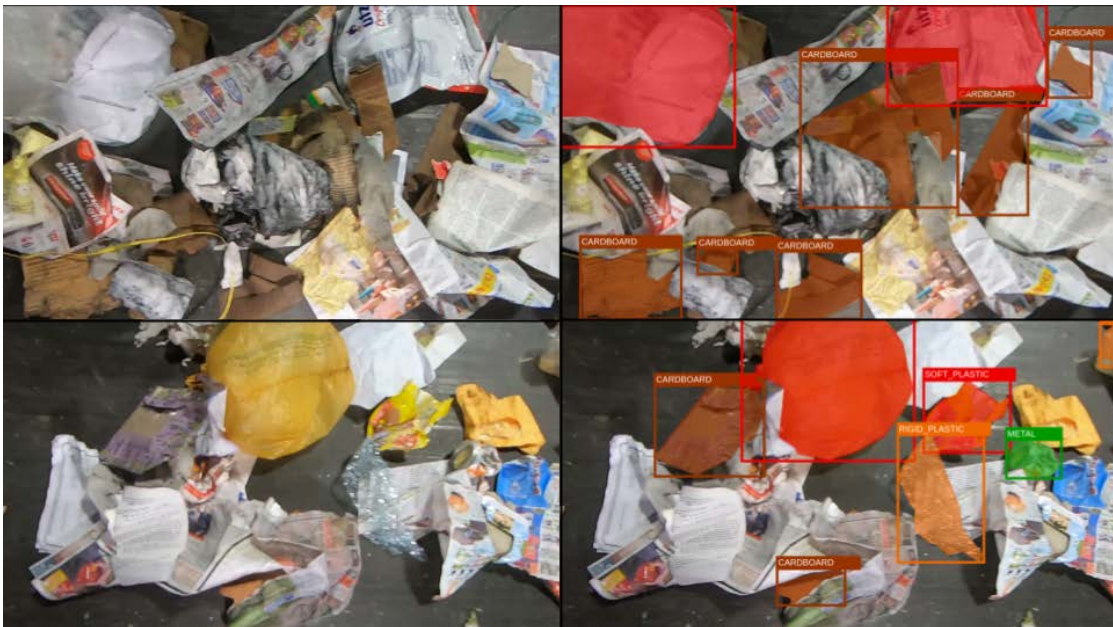
Figure 3.1: On the left, there is an example of two images extracted from the ZeroWaste dataset. The corresponding ground truth instance segmentation is displayed on the right [7].
