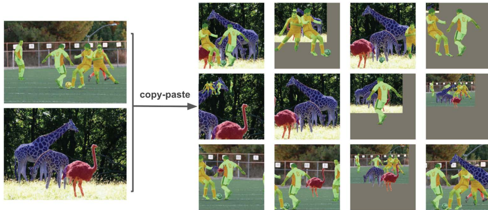
Figure 2.11: An example of Simple Copy-Paste augmentation [20]. Random scale jittering is applied on two random training images and then a subset of instances from one image is randomly selected to paste onto the other image.
