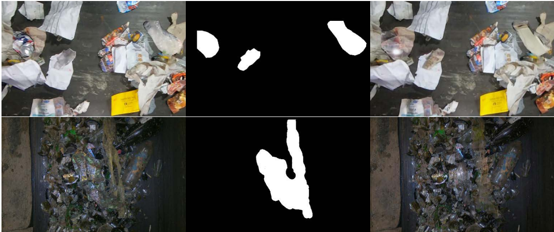
Figure 3.5: On the left the copy & paste version, on the center the segmentation mask and finally, on the right, the final harmonized result. Above an example from the ZeroWaste dataset, while below an example from the IT+Robotics-V dataset.
