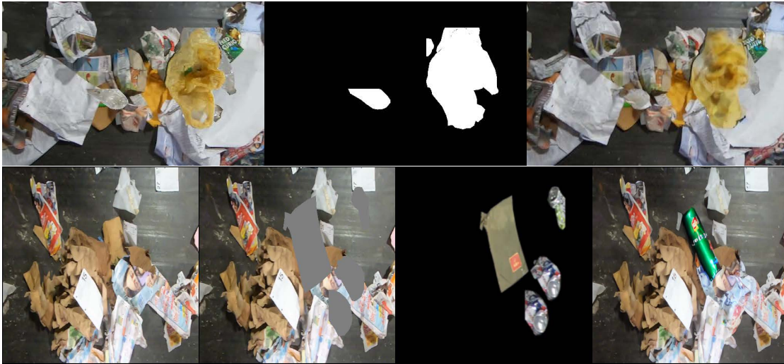
Figure 3.7: Above an example of the image harmonization approach where the lack of variety can be seen. Below an example from the image inpainting approach where you can see the limit in the mask-object correspondence.
