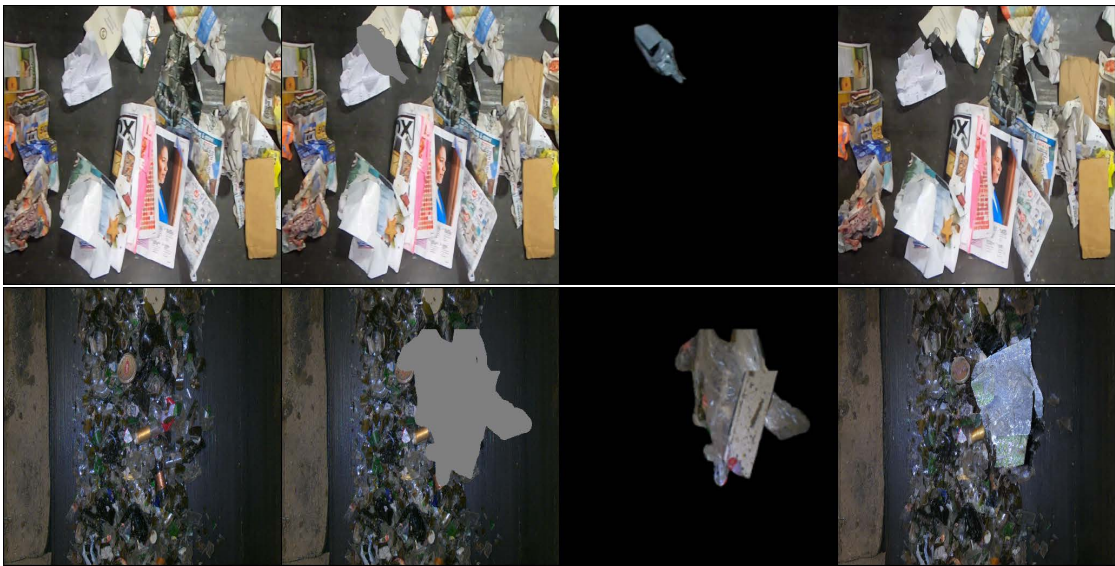
Figure 3.6: From left to right: the negative image (background), the segmentation mask of the patch to be inpainted, the reference patch and finally, the image inpainting result. Above an example from the ZeroWaste dataset, while below an example from the IT+Robotics-V dataset.
