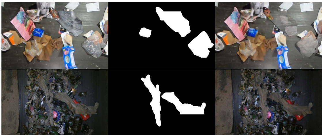
Figure 3.9: On the left the copy & paste version with the patch augmented by image inpainting, on the center the segmentation mask and finally, on the right the final harmonized result. Above an example from the ZeroWaste dataset, while below an example from the IT+Robotics-V dataset.
