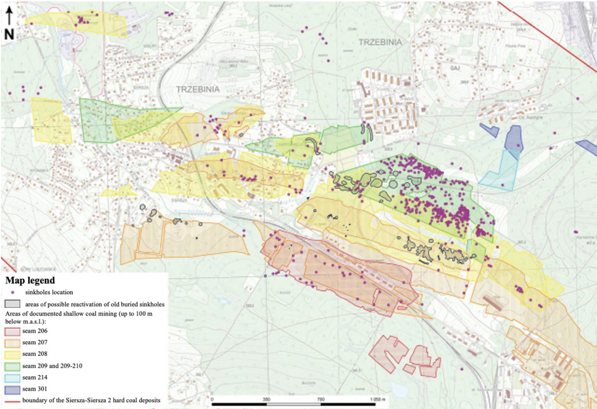
Figure 4.9 Area of highest concentration of sinkholes. Source: (Report on Analytical Work on Terrain Deformations in Trzebinia, Polish Geological Institute, 2023)
