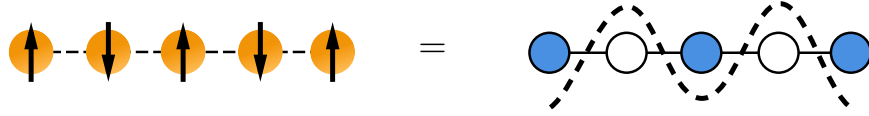
Figure 1.10: Equivalence between the antiferromagnetic ground state and the solution of a specific Maximum Cut problem.
