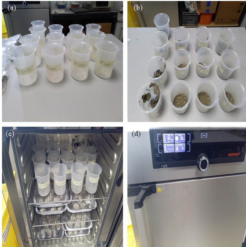
Fig. 13 Drying step of soil samples collected from the field: (a) Labelling each soil sample by depth using beakers; (b) Weighing 50 g of each soil sample; (c) Placing the prepared samples in a cool oven for drying (Note: The soil samples visible on the lower shelves of the cool oven belong to another researcher); (d) Setting the cool oven to 60 °C and initiating the drying process (photos by O. Şahin).
