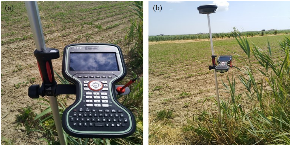
Fig. 9 The process of determining the coordinates of soil sample points using GPS technology: (a) The GPS device utilized for marking sampling locations, and (b) The initial setup of the GPS device to establish the reference point.
