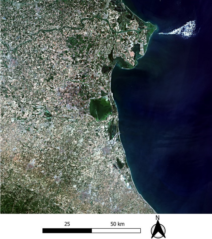
Fig 19 Natural colour composite (RGB: 432) of virtual raster created using Sentinel-2A imagery data
