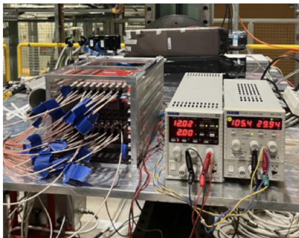
Figure 7.3: Photo of the DAQ system used for the test beam. On the left, the rack containing the Mezzanine electronics boards along with two digitizers is visible, while on the right, the power supply system is shown.
