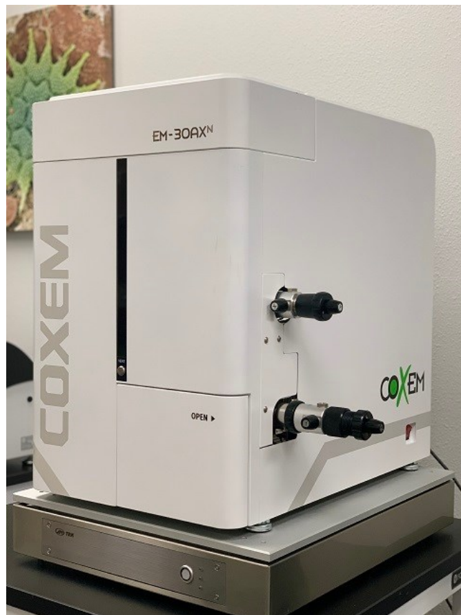
Figure 13 COXEM EM-30AX Tabletop SEM with STEM detector at Insertion position using the side accessory port
