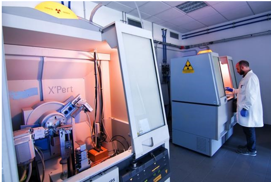
Figure 12 Philips X'Pert PRO diffractometer, Bragg-Brentano geometry with Bragg-Brentano HD optics, cobalt source, X'Celerator detector, and Anton Paar HTK16 hot stage. (source: https://www.geoscienze.unipd.it/diffrattometria-x-polveri )
