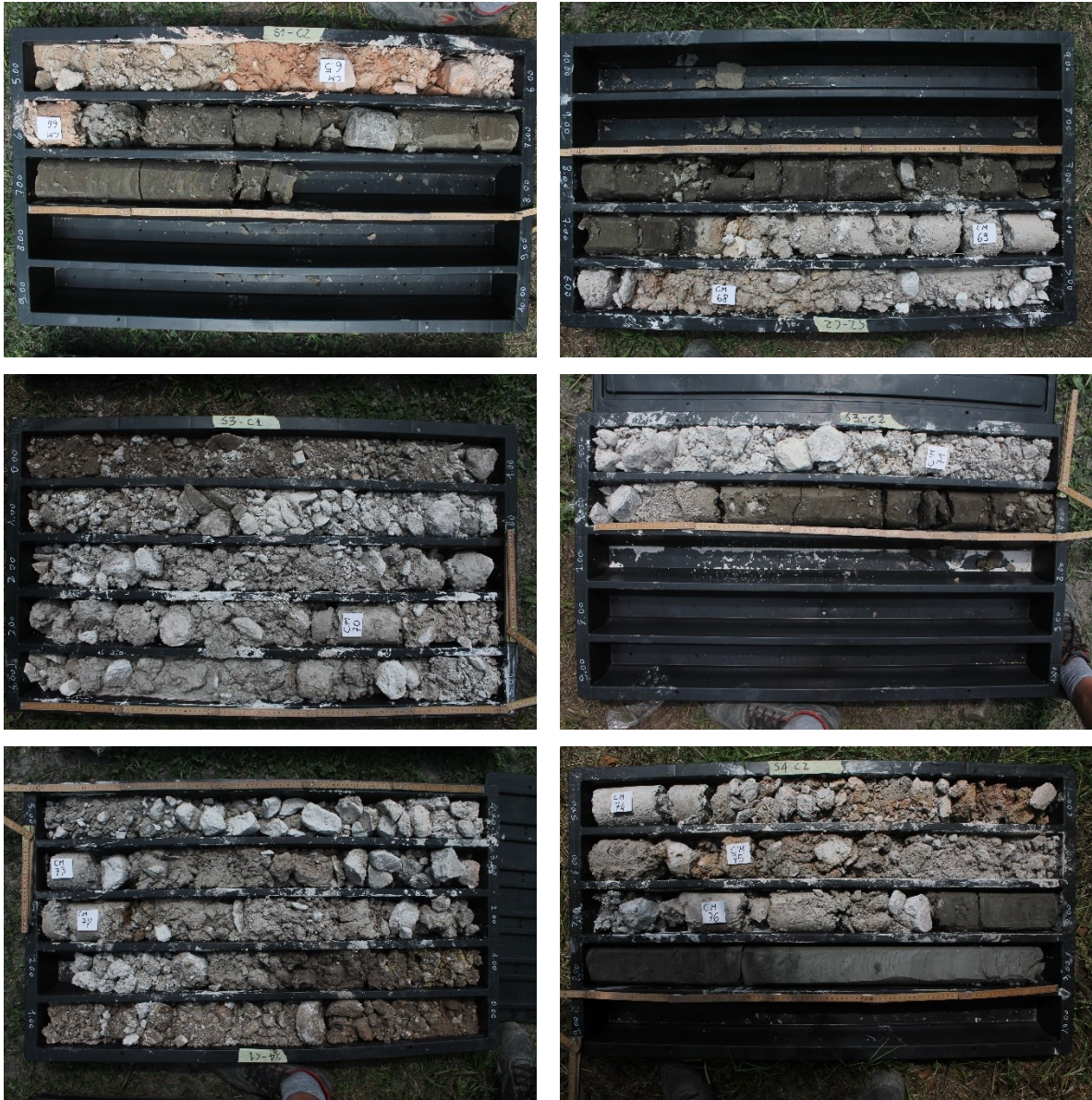
Figure 9 Core drills from the foundational layer with sampling points and their relative heights
