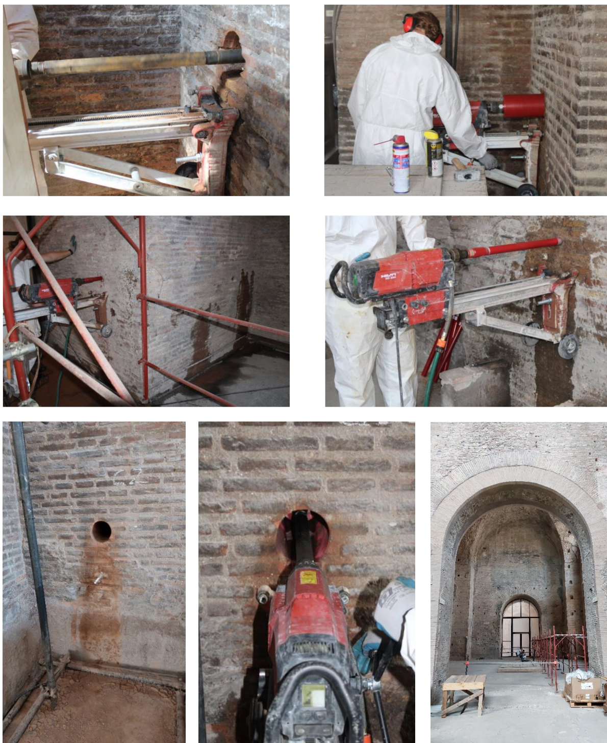
Figure 10 Sampling process at the Basilica of Santa Maria degli Angeli (Source: SO.IN.G. strutture e ambiente S.r.l.)
