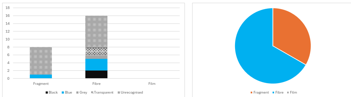
Figure 36: Microplastic distribution for sample A-39. The colour distribution of different shapes (left) and the proportions of different shapes in the sample(right)
