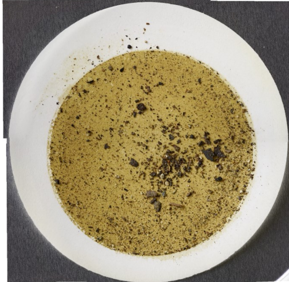
Figure 14: An example of a high-resolution photo of the filter paper containing the microplastic particles along with some debris.
