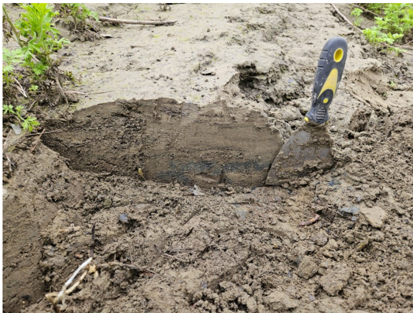
Figure 98: Closeup of the sampling location, the freshly deposited sand is distinguishable from the bud below.
