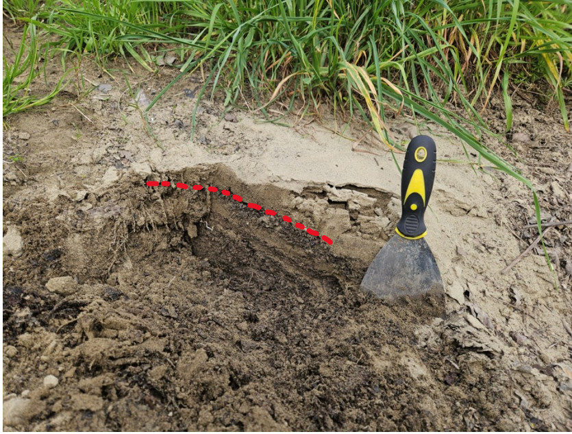
Figure 10: Sampling site (A-25), The red line shows the lower boundary of the fresh sediments deposited during the most recent flood. The material below has roots, meaning it was deposited much earlier, allowing biological activity to take place.
