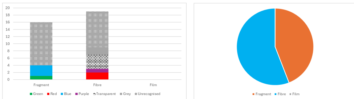
Figure 80: Microplastic distribution for sample A-16. The colour distribution of different shapes (left) and the proportions of different shapes in the sample(right)
