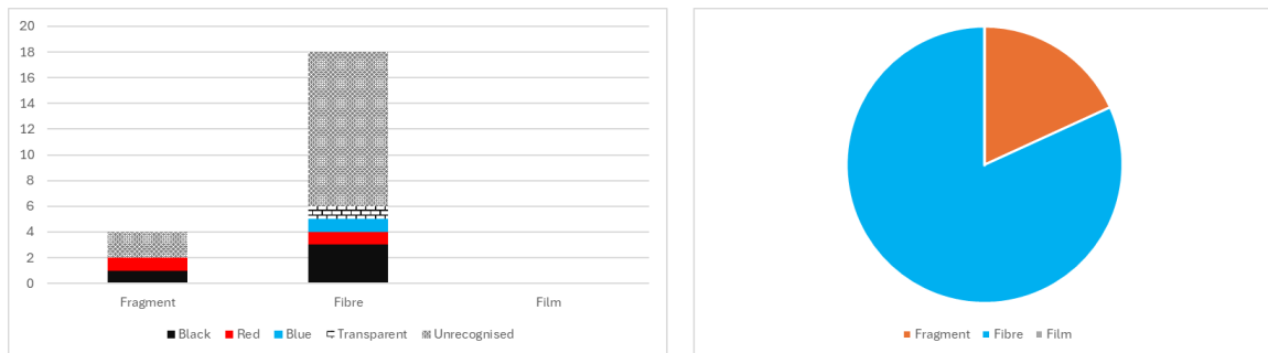
Figure 45: Microplastic distribution for sample A-33. The colour distribution of different shapes (left) and the proportions of different shapes in the sample(right)
