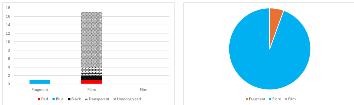
Figure 24: Microplastic distribution for sample A-46. The colour distribution of different shapes (left) and the proportions of different shapes in the sample(right)
