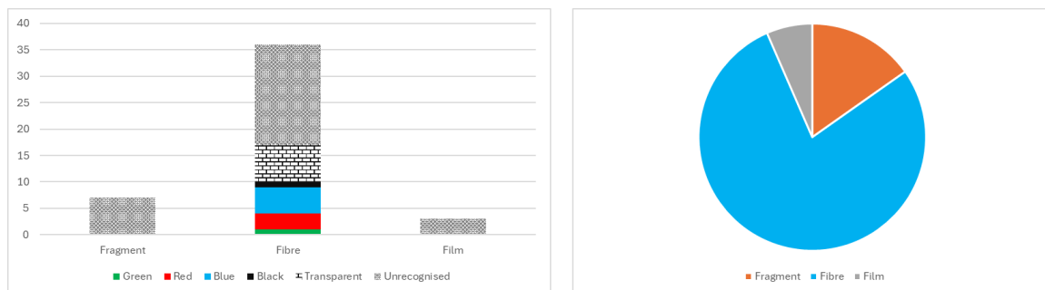
Figure 83: Microplastic distribution for sample A-14. The colour distribution of different shapes (left) and the proportions of different shapes in the sample(right)
