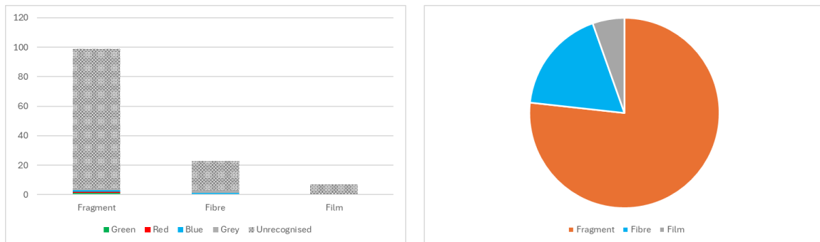
Figure 103: Microplastic distribution for sample A-2. The colour distribution of different shapes (left) and the proportions of different shapes in the sample(right)
