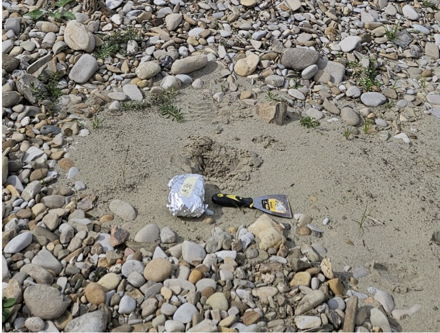
Figure 11: The samples were collected using a metal shovel and packed in aluminium foil to avoid contamination.
