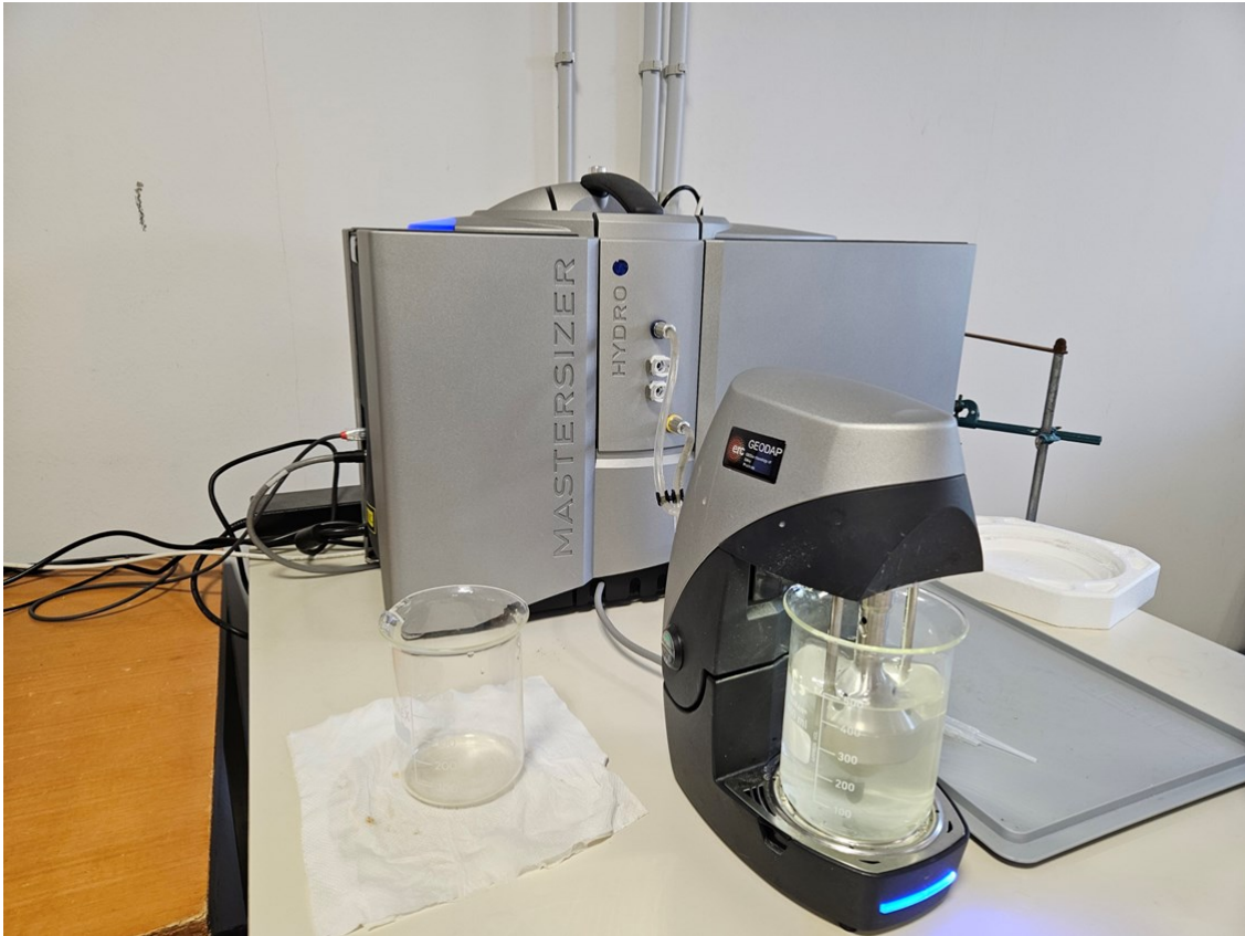
Figure 12: Image of the Mastersizer 3000, used for grain size analysis. The wet dispersion unit in the front and the Optical unit at the back.
