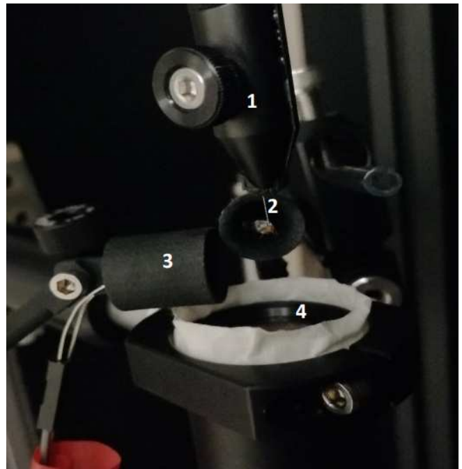
Figure 4.3: 1) Micromanipulator; 2) Needle+Fly system; 3) LED spotlight; 4) Ximea Camera's lens.
