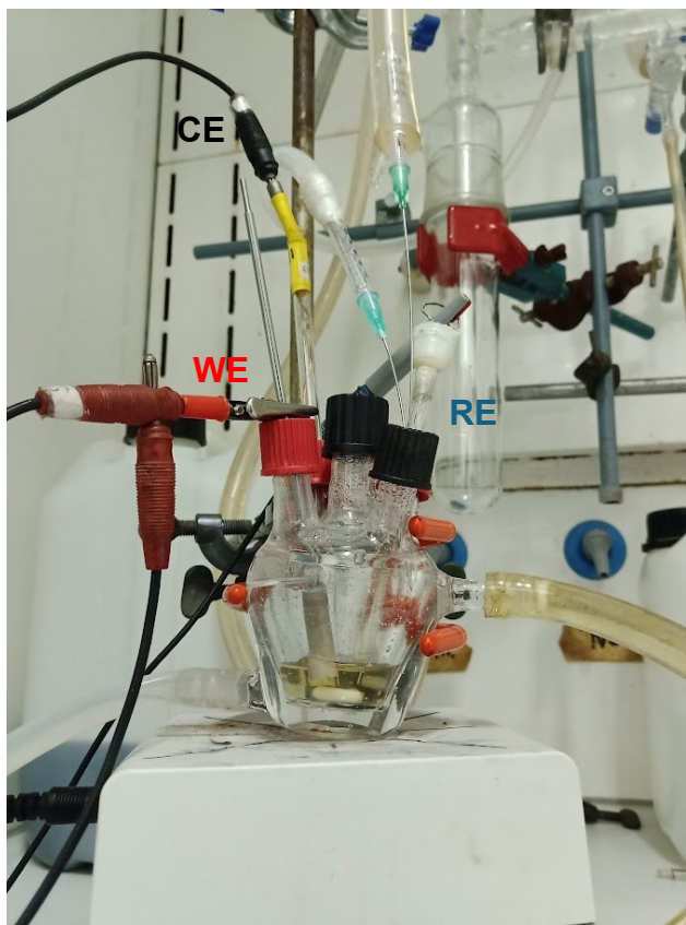
Figure 31 Typical CV experimental setup, with WE: glassy carbon electrode; CE: platinum wire electrode; RE: Ag/AgI separated cell electrode
