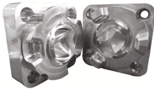
Figure 4.1. Aluminium mould inserts for the J6 valve [124].
