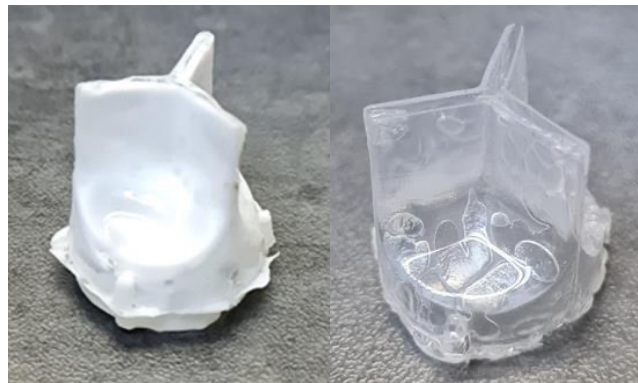
Figure 4.4. Two valve prototypes fabricated with polyurethane: the valve on the right shows how the compression speed has a role in developing and entrapping air bubbles [135].
