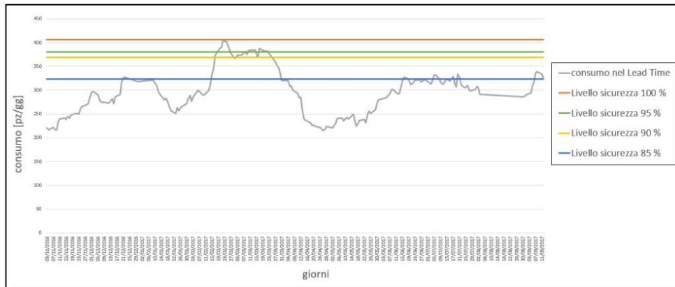
Fig. 4-6 Variation in the average daily consumption to be considered when calculating the number of kanban based on the safety level chosen
