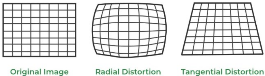
Figure 6: Radial and Tangential distortion
