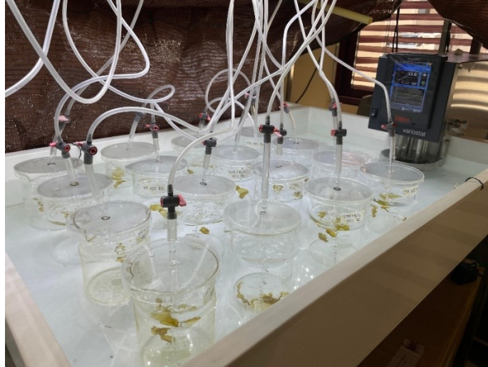
Figure 13 - Temperature controlled water bath for one temperature treatment. Each 1 L aerated glass beaker contained 4 sporophytes.
