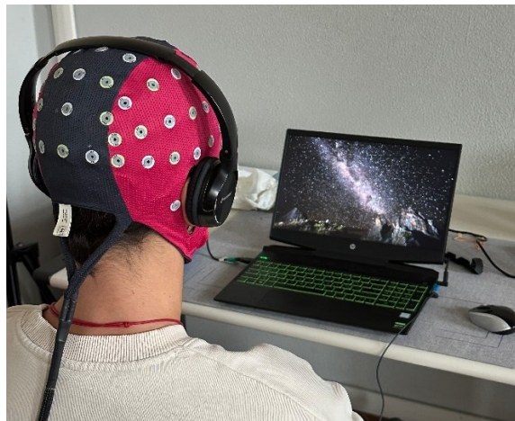
Fig. 2.2: Picture taken during the experiments in the laboratory showing a subject under auditory NFB. In the picture is shown the EEG cap with 64 electrodes, an image shown at screen and headphones for auditory feedback.
