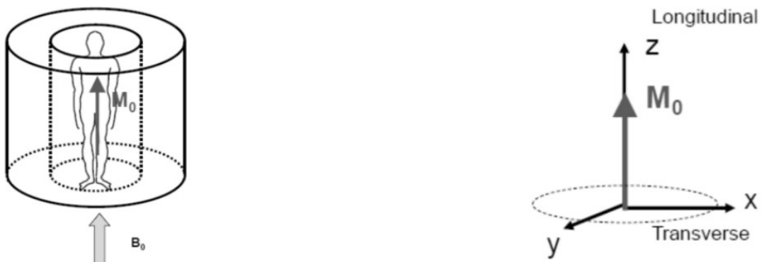
Figure 2: MRI Reference System. M_0 , or B_0 , is the static magnetic field. The reference system is organized in such a way that the z axis coincides with the direction and direction of B_0 (or M_0 ), while the x and y axes lie on a plane perpendicular to z
