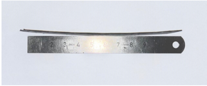
Figure 4.8: Bending after grinding half the thickness of the sample.
