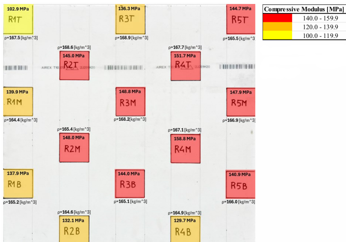
Figure 4.19: Results Mapping over the panel
