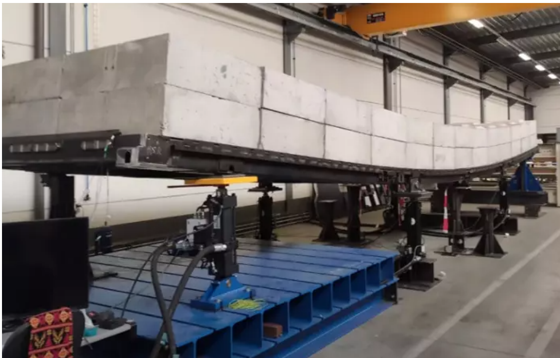
Figure 1.2: True-scale testing of the container's floor. Courtesy of AGESIA.
