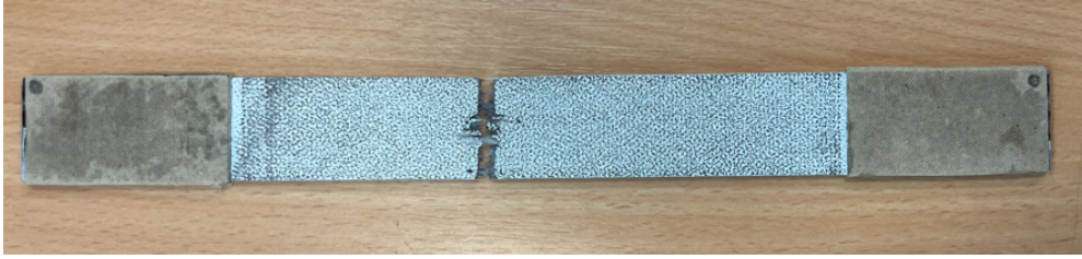
Figure 3.11: Broken specimen, with speckle pattern and tabs
