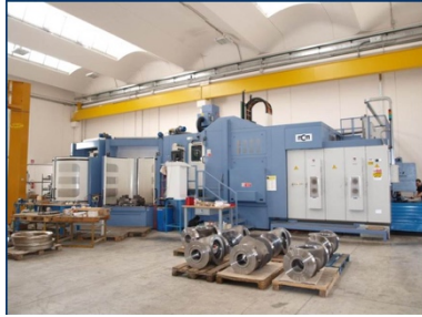
Figure 22: M.C.M Machining Centre for valves up to 30"
