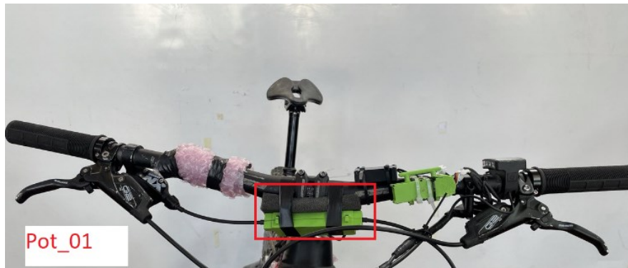
Figure 2.5: linear potetiometer placement on the bike
