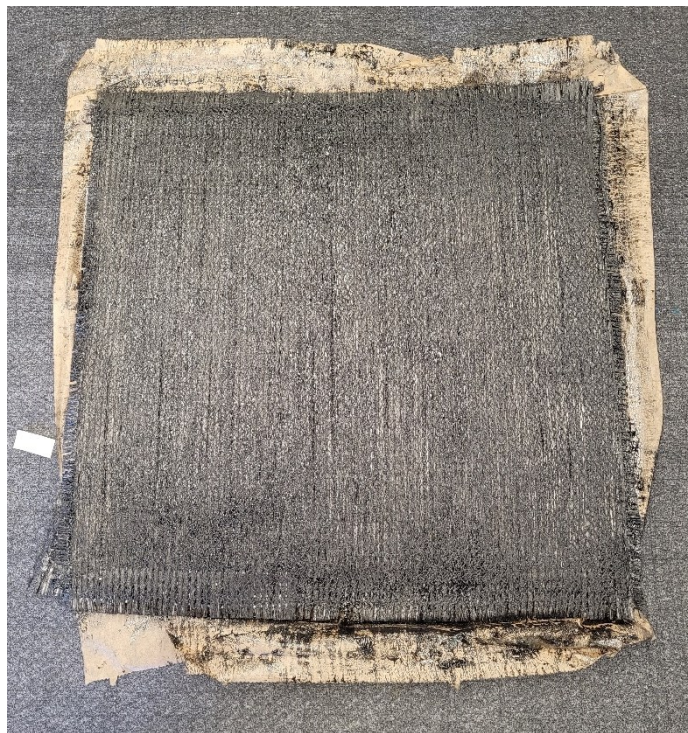
Figure 2.4 - Plate hand laminated with modified resin during the lamination process.
