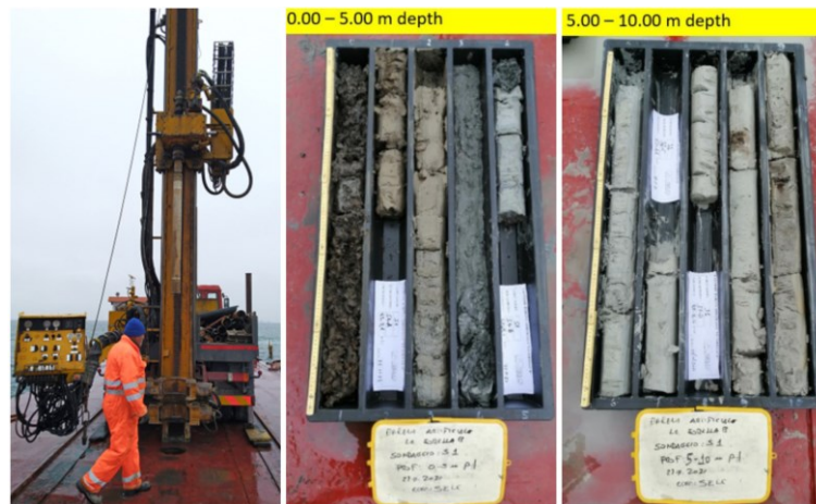
Figure 2.13. The drilling machine used in coring procedure and cataloging boxes at relative depths. The empty zones indicate the undisturbed specimens collected for the oedometer tests (Meneghini, 2022).
