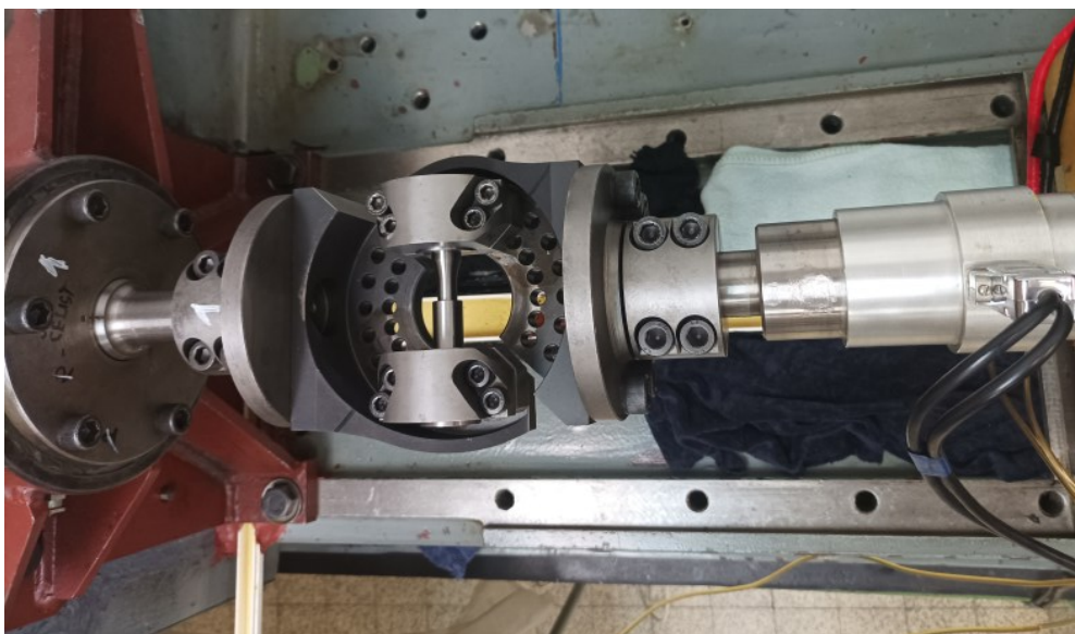
Figure 3.5: Another of the same specimen ready to be tested under plane bending load.
