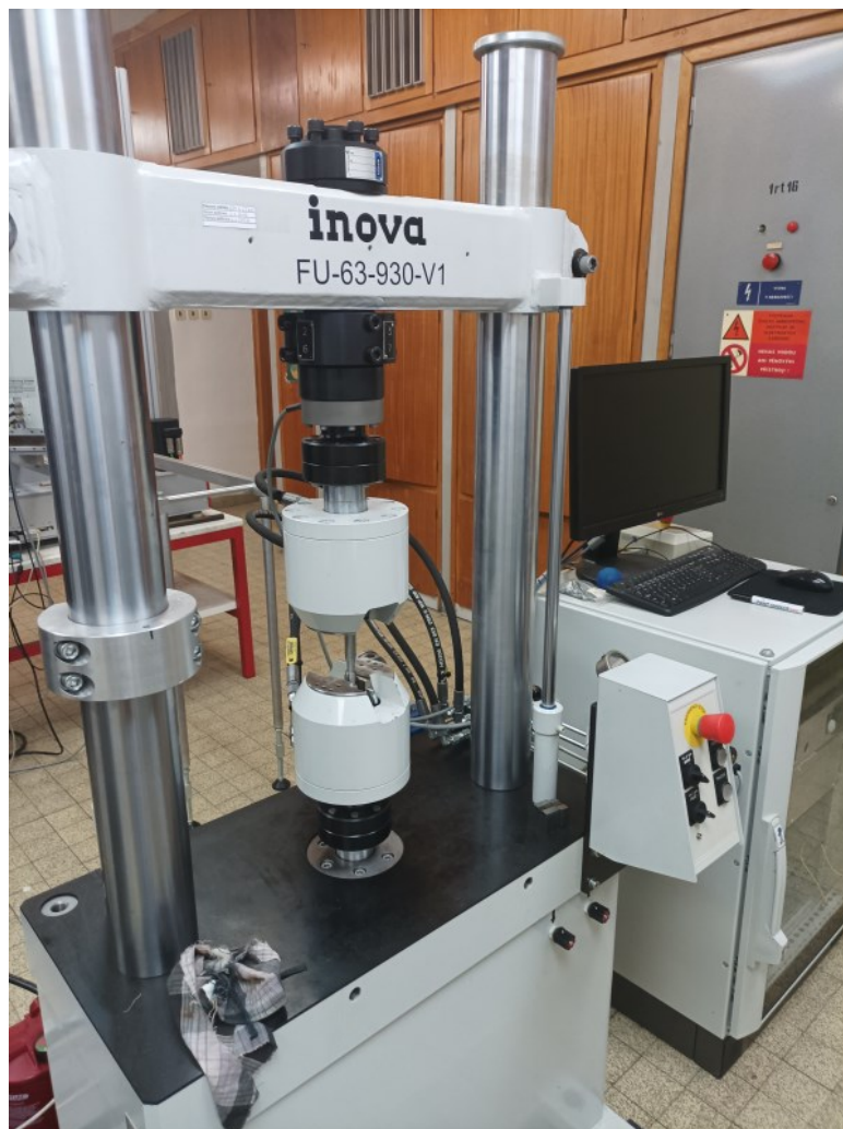
Figure 3.1: INOVA FU-63-930-V1 machine used for push-pull tests.
