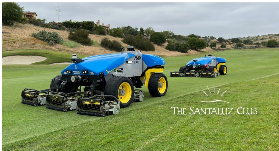
Figura 52: tosaerba autonomi della ditta Firefly Automatrix impiegati al The Santaluz Club a San Diego, California ( https://fireflyautomatrix.com/amp-mowers/ )
