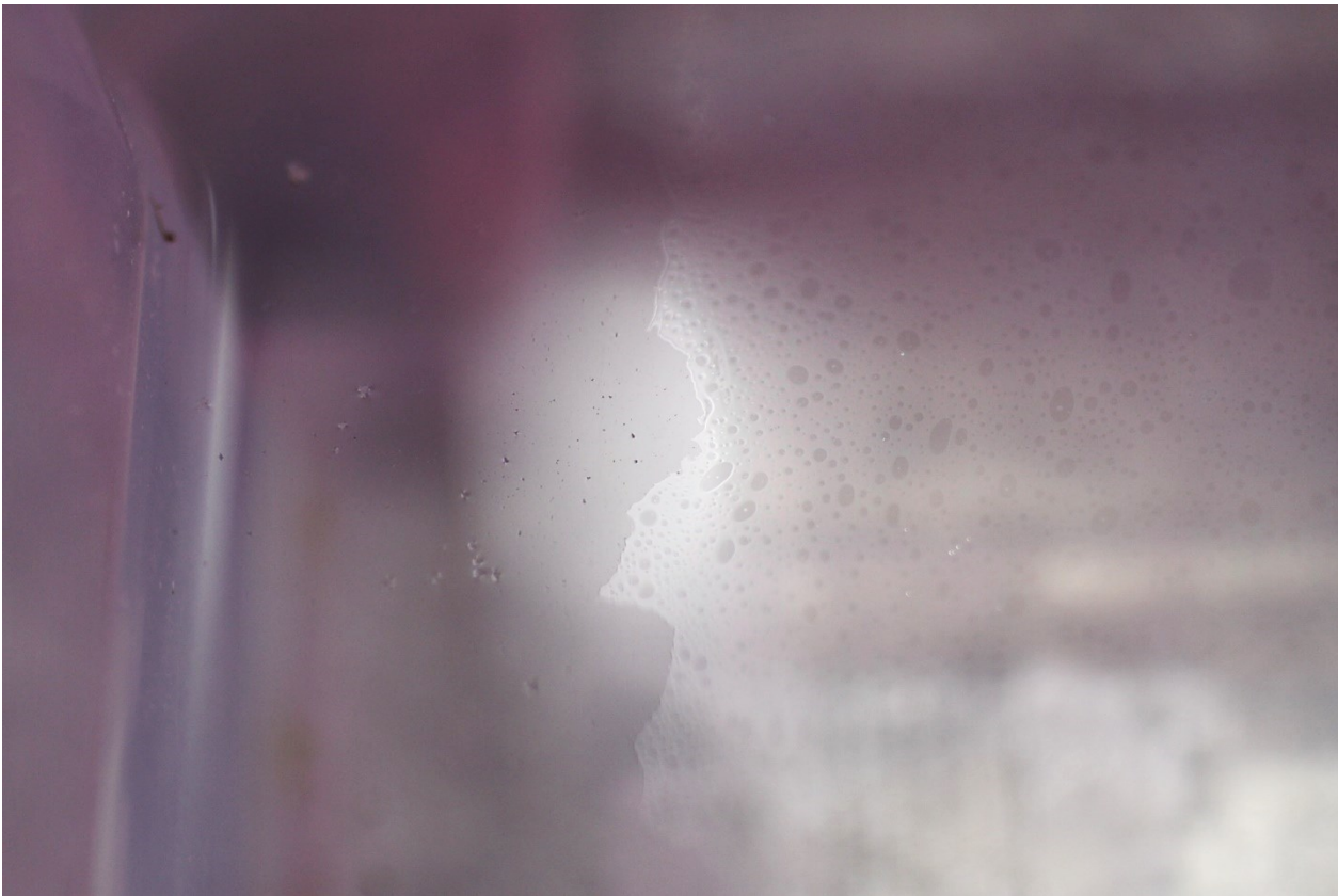
Figure 4.6: limited spreading of Aquatain AMF layer at 28 µL dose
