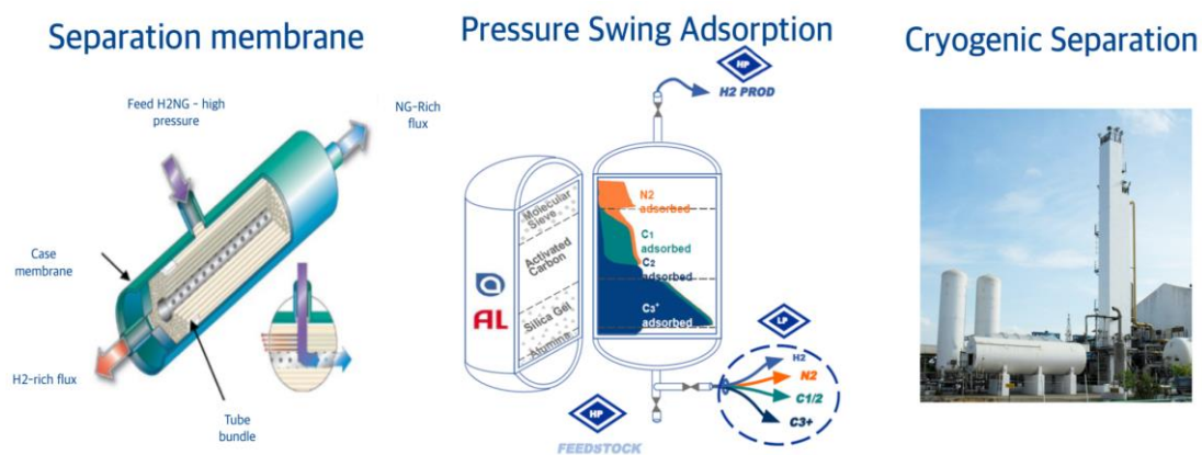
Figure 11- Graphical representation of different methods for the separation of natural gas and hydrogen mixture.
