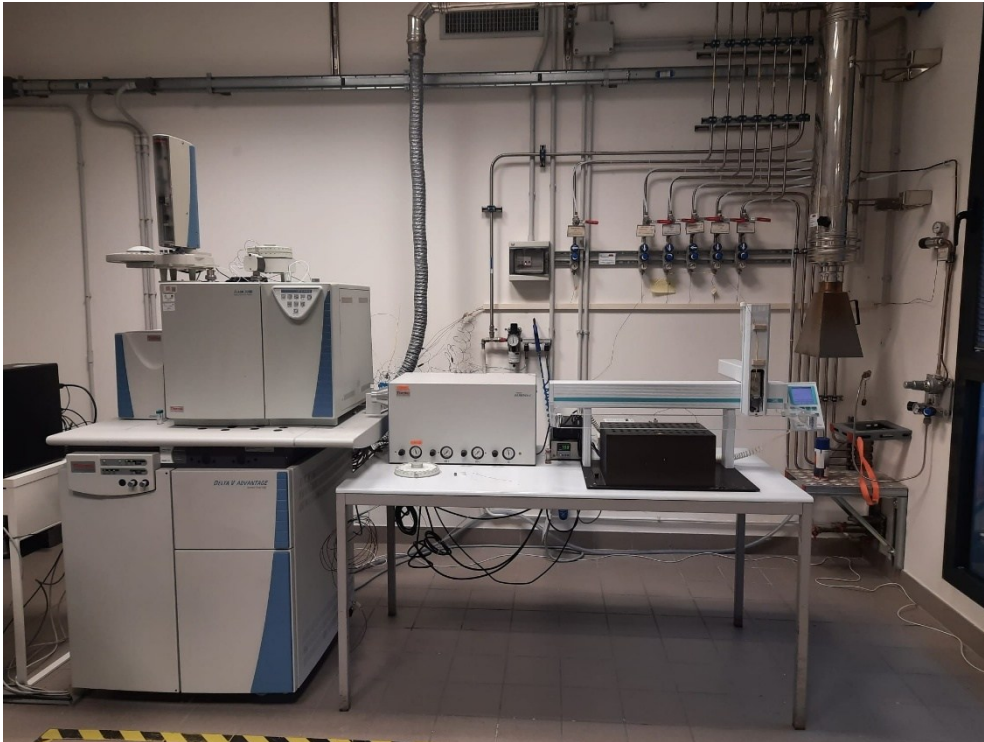
Figure 7. Thermo Delta V Advantage isotope ratio mass spectrometer (IRMS) at the Department of Geosciences, University of Padova, which was used during the analysis.
