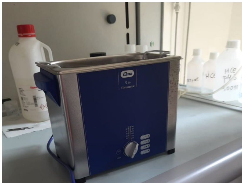
Figure 10. The Elmasonic ultrasonic cleaner is used in order to remove the contaminants from the etched samples.
