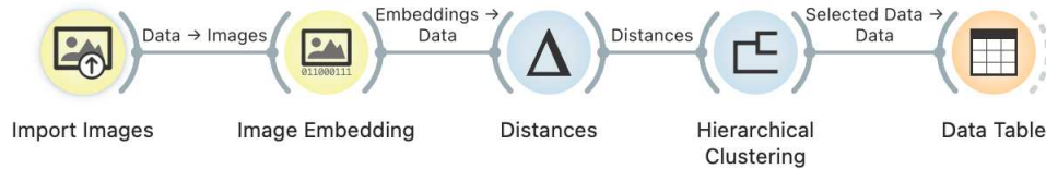
Figure 2.3: Workflow that performs clustering analysis on images
