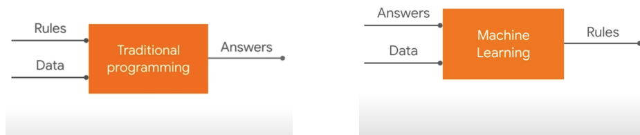
Figure 2.1: Comparison between Traditional programming approach and machine learning: (a) Traditional programming framework, (b) Generic machine learning framework.
