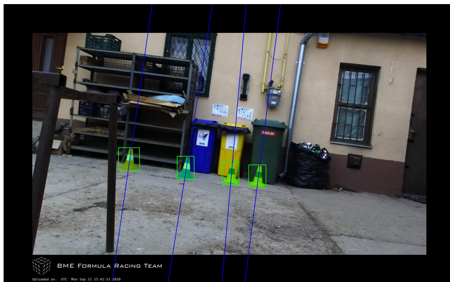
Figure 5.5: Example of cone peak extraction with a not horizontal horizon. Cone segmentation is visible in green, in blue the principal axis and in red the final cone peak.
