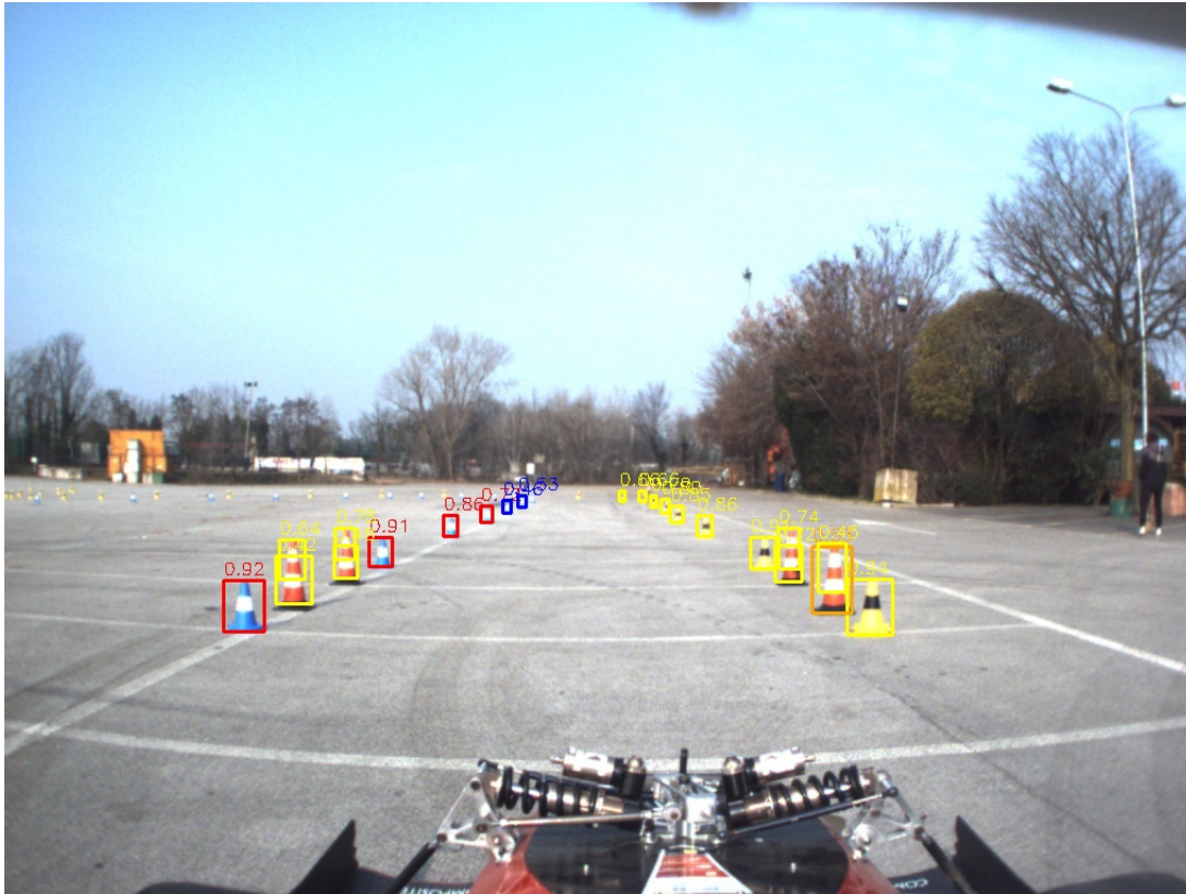
Figure 5.1: Example of fine-tuned yolov7 inference on an image of the data acquisition described in 4.1. 3 big orange cones are classified as yellow and 4 blue cones are classified as small orange.
