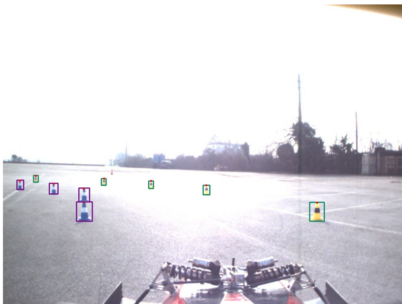
Figure 5.8: Result of the YOLO11-Pose fine-tuned on a data acquisition image, note that the model detects cone even in harsh lighting conditions.
