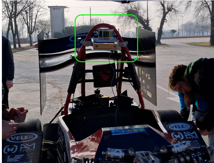
Figure 4.1: Sensor placement for the first data acquisition
