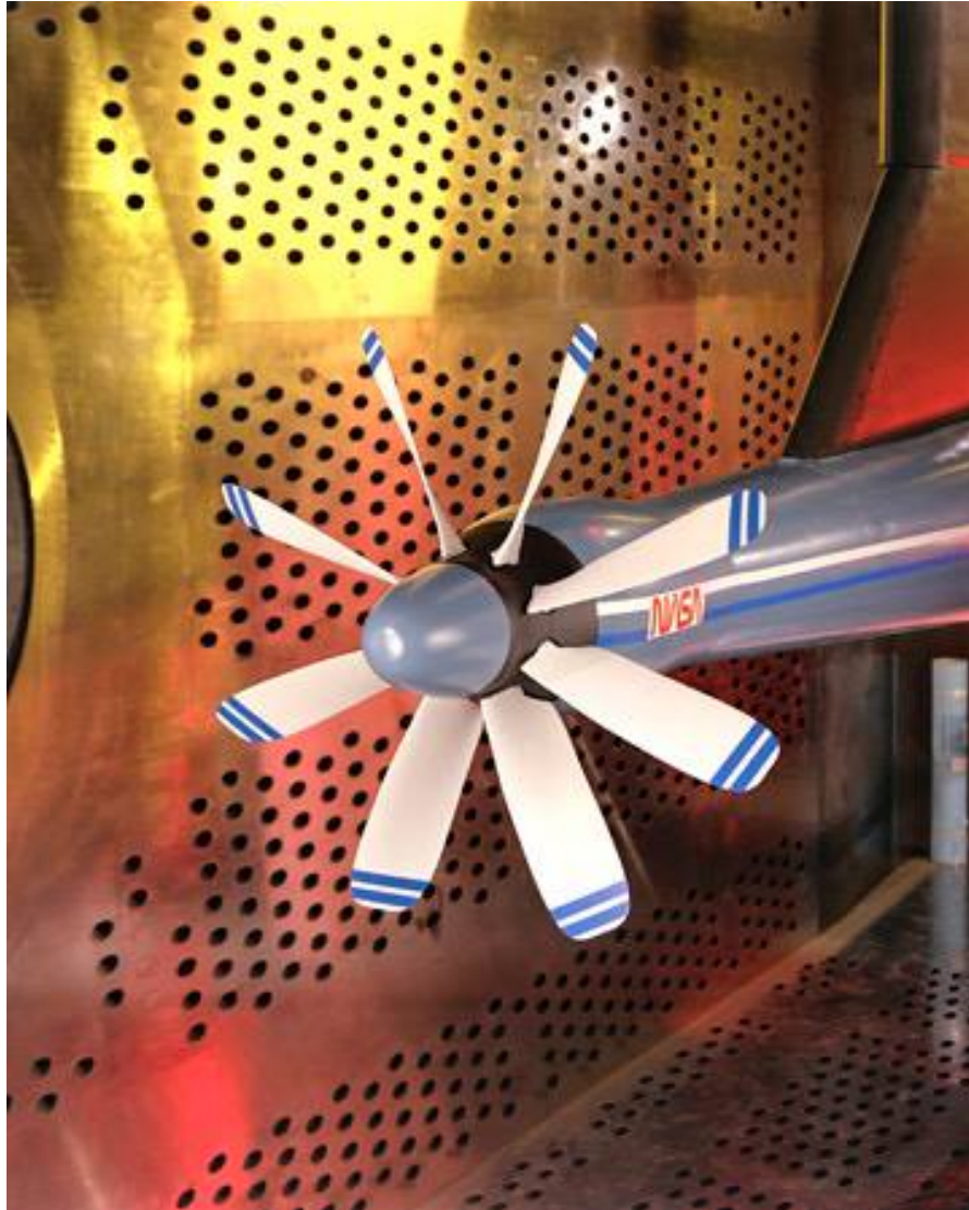
Figure 1.7: SR2 propeller model inside NASA wind tunnel
