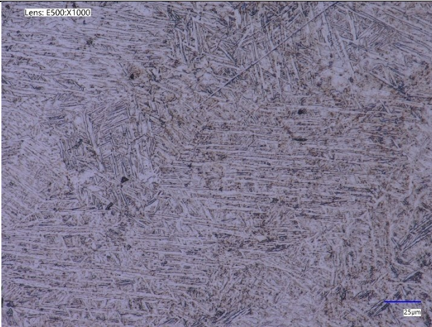
T = 950°C, \epsilon = 10 \text{ s}^{-1} horizontal build, building direction
