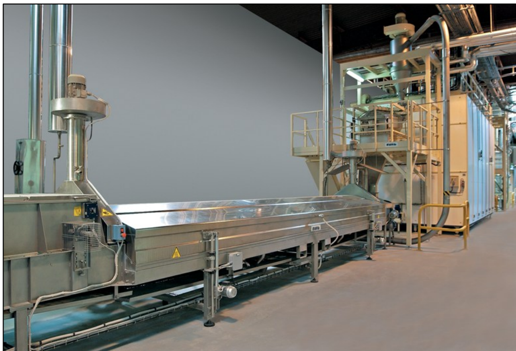
Fig. 4.34 Couscous line from the cooker to the dryer [3]
