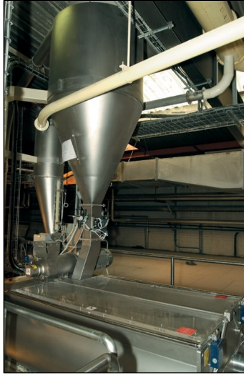
Fig. 4.35 Mixing tank and cyclones of the couscous production line [3]
