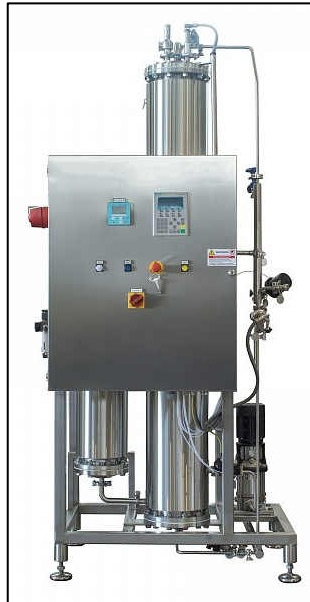
Fig. 4.66 Pure steam generator used for sterilization and disinfection in the food industry [25]
