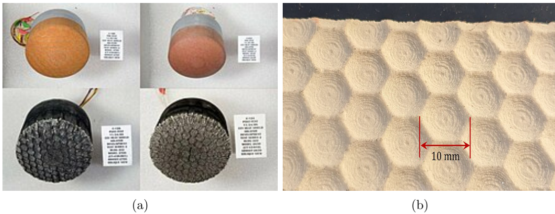
Figure 3: (a) Apollo and Orion ablative heat shields before and after testing (credit: NASA). (b) Example of a thermal protection roughness structures (image from Miller et al., 2024).
