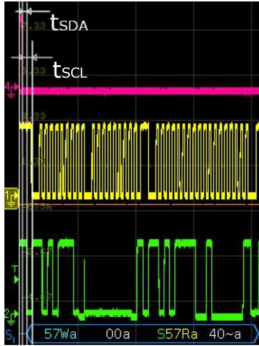
Figure 3.6: Times required by the I2C to start
