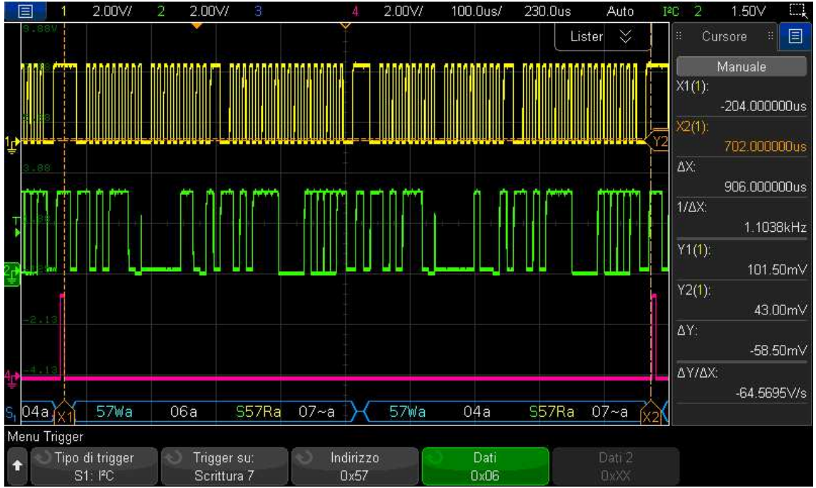
Figure 3.5: Complete loop cycle in case of no data found in the sensor's FIFO for the check logic ( t_{loop\_data\_check} )
