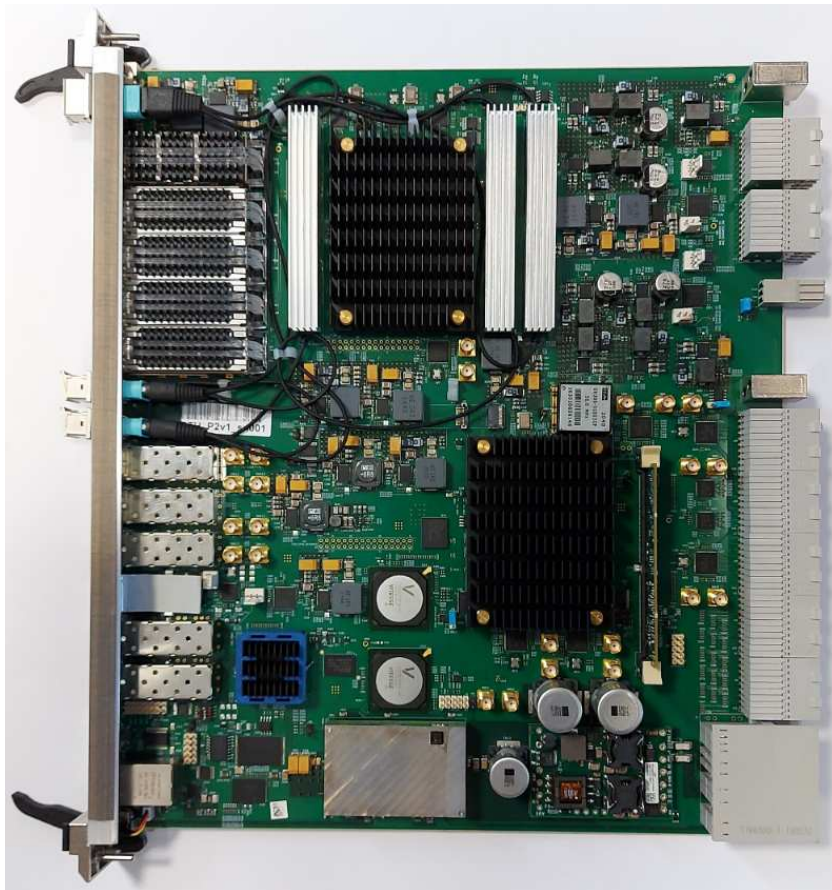
Figure 3.3: Image of the DTH-400 board. The CMS DAQ FPGA is under the top black heat sink.
