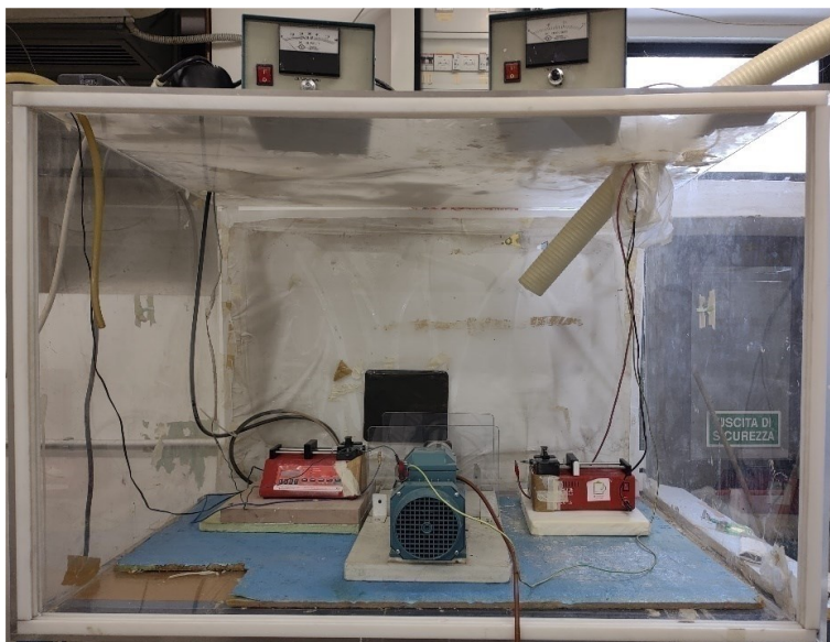
Figure 3.2. Setup for a simultaneous electrospinning
