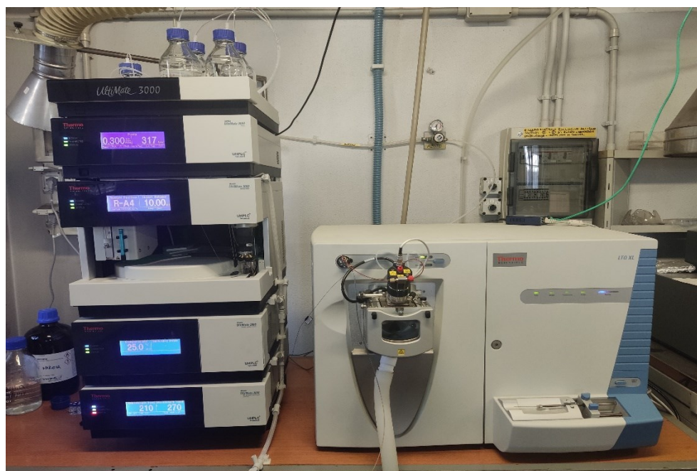
Figure 3.9. Ultimate 3000 UHPLC system coupled with MS Thermo scientific LTQ XL
