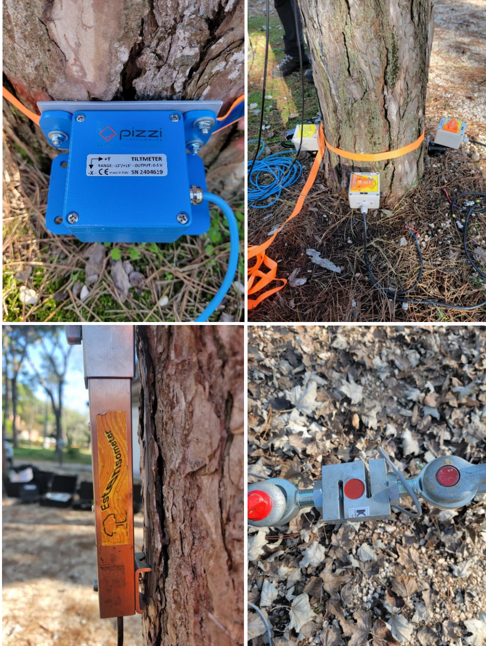
Figure 1. The supplementary sensors used in this study to collect and verify data. This study utilized, in addition to the principal sensor array, two tiltmeters (top left), three inclinometers (top right), two elastometers (bottom left), and a tensiometer (bottom right).
