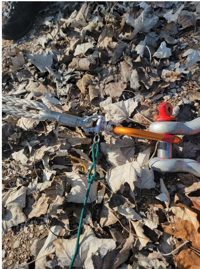
Figure 4. The quick-release mechanism installed in place of the tensiometer for the pull-and-release tests.
