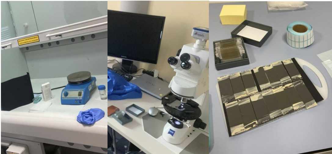
Figure 3.4: Laboratory workflow for calcareous nannofossil analysis. From left to right: sample preparation under fume hood with precision scale and tools; observation under a Zeiss polarizing microscope; prepared smear slides organized and labeled for analysis. Photos taken at the Department of Geosciences, University of Padova.
