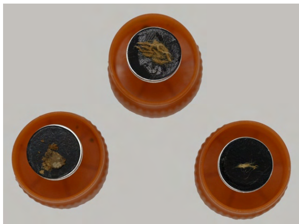
Figure 12: 3 of the textile fragments, affixed with adhesive tape on aluminium mounting stubs. Photo by E. Faresin.
