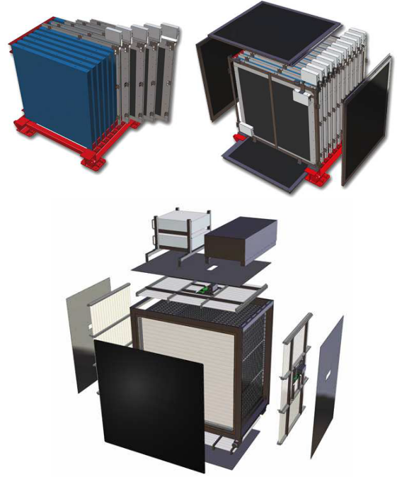
Figure 2.7: Models of an INGRID module (top) and a proton module (bottom).
