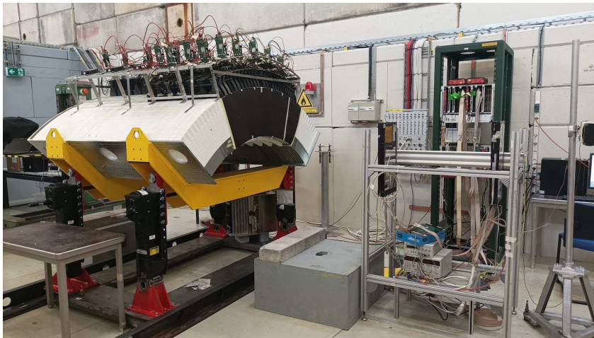
Figure 1.9: The ENUBET demonstrator (1.65 m length, 3.5 t mass). From [23].
