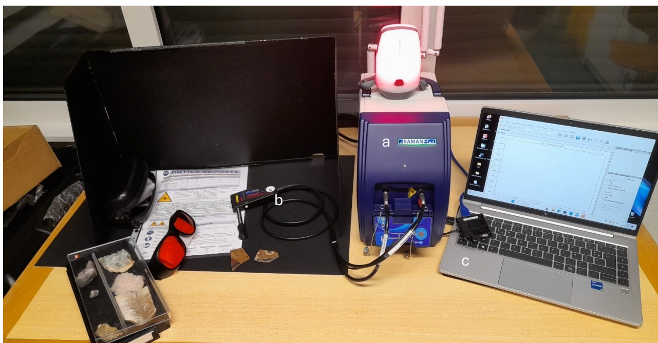
Figure 20. BWTEK i-Raman Plus 532s Raman spectrometer set up, showing (a) the power supply unit, (b) the optical fiber probe for laser delivery and signal collection, and (c) the laptop with dedicated software for data acquisition (Sifatullah Hassin).
