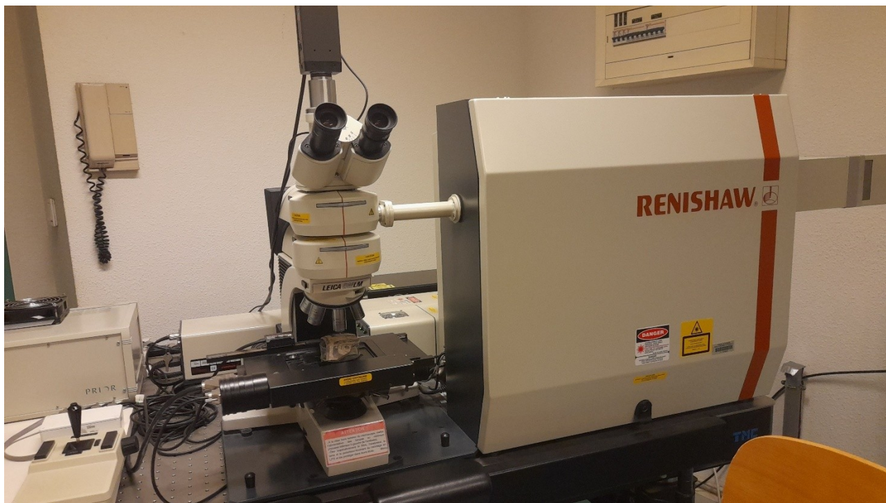
Figure 21. Benchtop Raman spectroscopy performed with 532 nm, 633 nm, and 785 nm laser excitations (Sifatullah Hassin).
