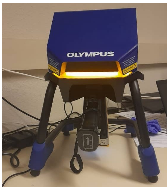
Figure 19. Olympus Vanta XRF analyzer mounted on a fixed lab stand used for the analysis (Sifatullah Hassin).
