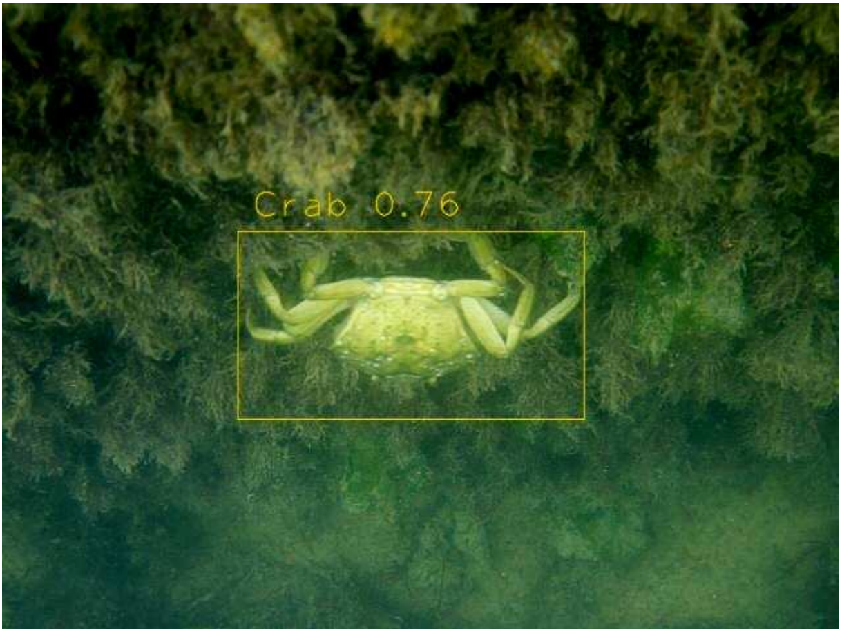
Figure 3.2: Crab detected by the CV algorithm.
