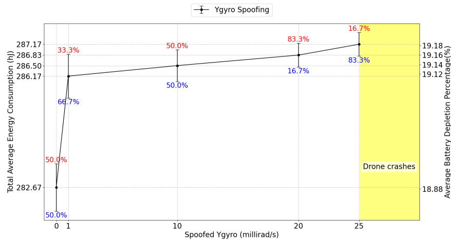
(b) Impact of spoofing the Ygyro sensor values of all three available gyroscopes.
