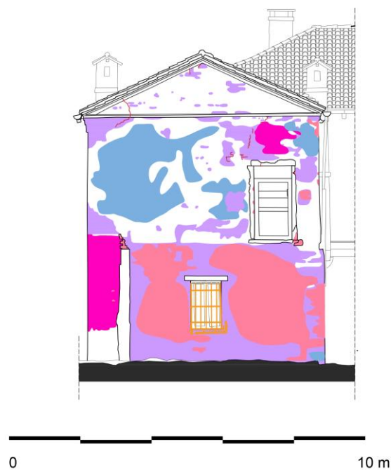
Figure 52. Damage map of the second easy (E2) façade of the Generalato.
