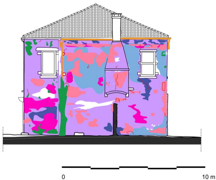
Figure 49. Damage map of the north (N1) façade of the Generalato.
