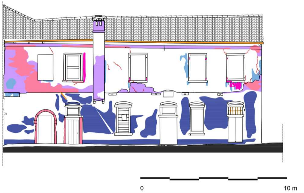
Figure 48. Damage map of the south (S) façade of the Generalato.
