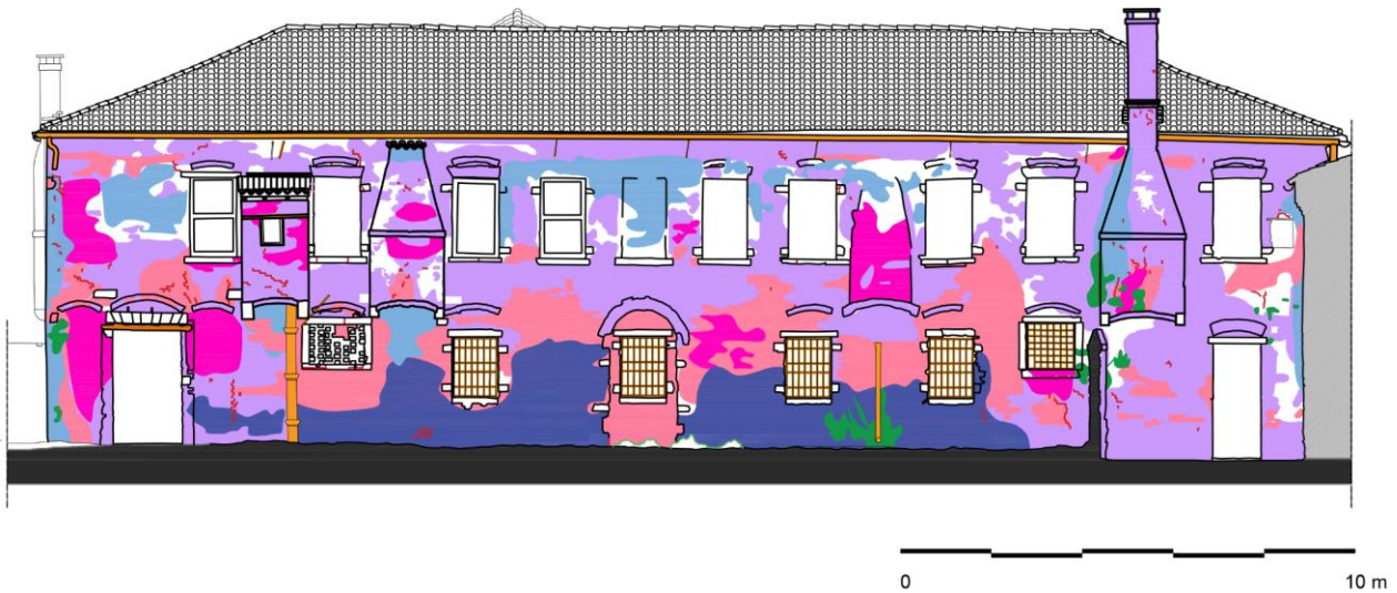
Figure 47. Damage map of the west (W) façade of the Generalato.
