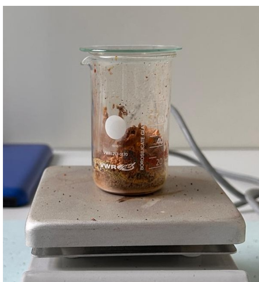
Figure 2.8: Auto-Combustion reaction, ignition of the flame.
