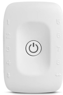
Figure 3.1: BiosignalsPlux device used for multimodal physiological signal acquisition.
