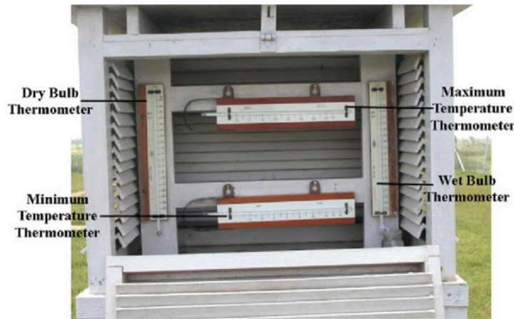
Figure 3.14: Picture and schematic illustration of a Stevenson screen [50].
