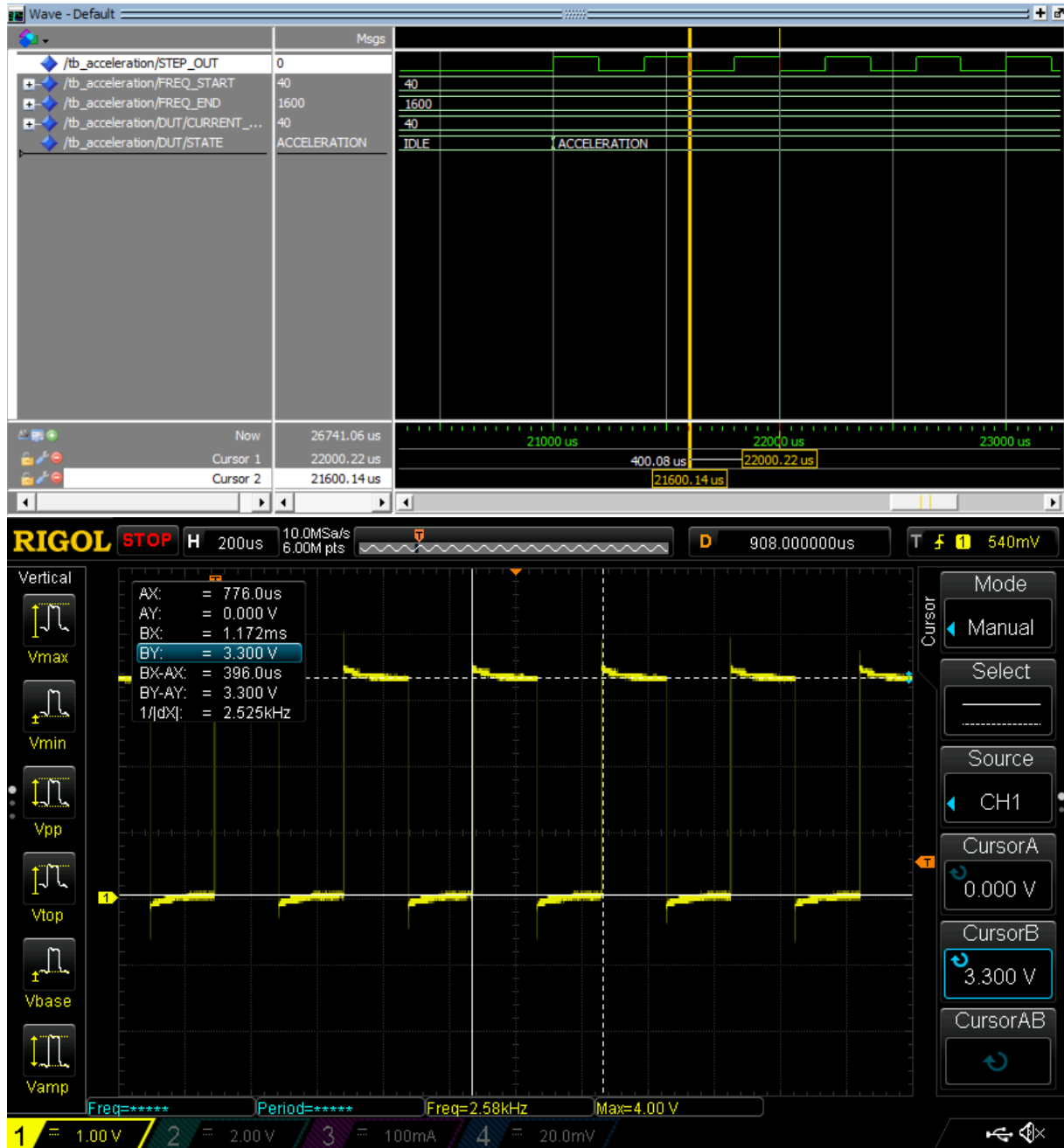
Figure 7.3.2: Comparison between simulation and experimental results at the minimum frequency.
