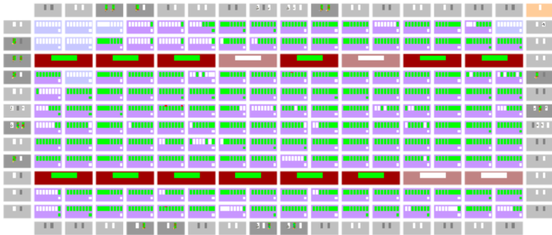
Figure 6.1.1: Visual representation of the total resources used. LUTs in green, PLBs in blue, RAM in red.
