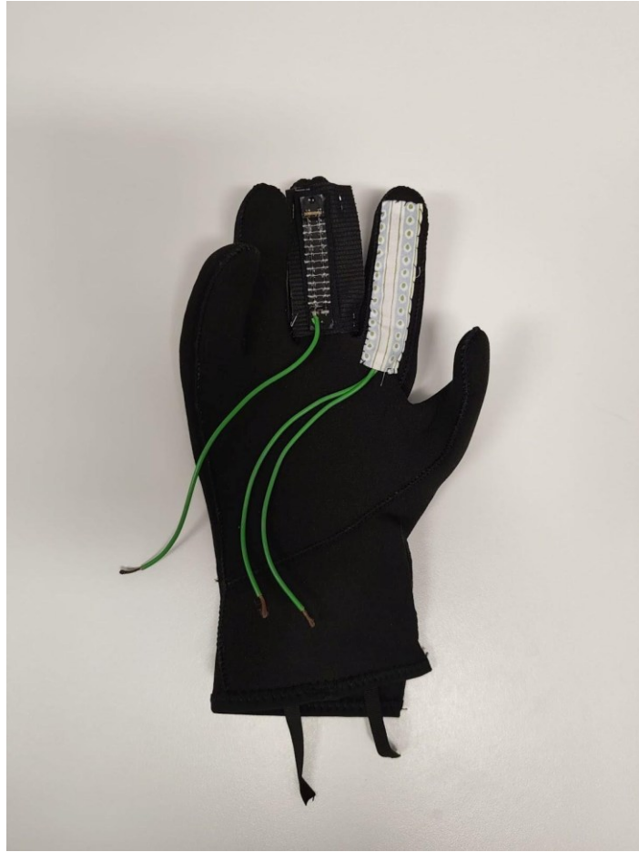
Figure 18 removable (on middle) and stable (on index) integration on the palm of the hand
