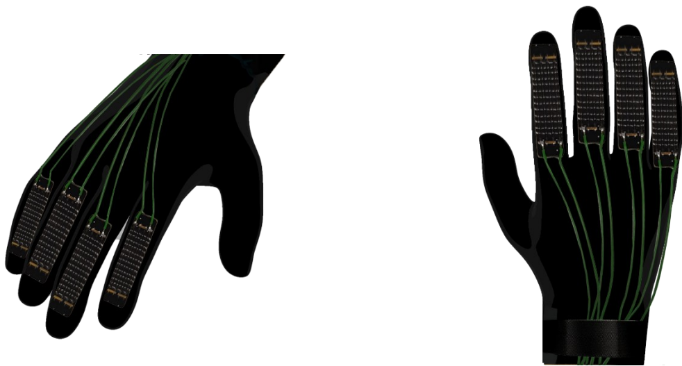
Figure 14 3D rendering of the back of the hand with hypothetical SMA actuators
