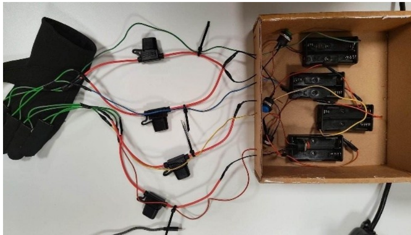
Figure 22 final prototype with power supply and control system
