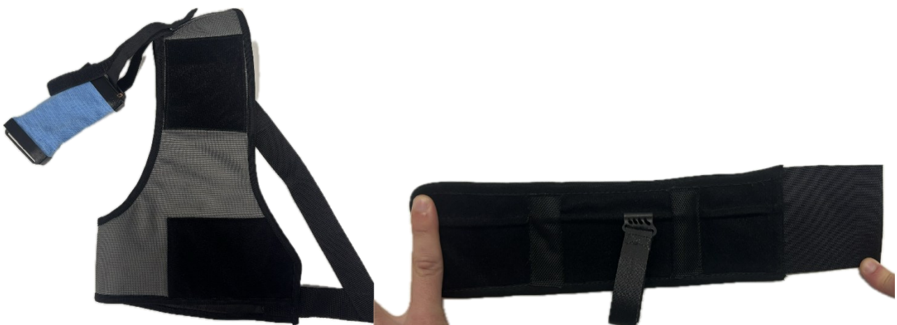
Figure 34 Details of the torso part (left) and the armband (right): the cordura is visible in grey and the velvet in black, intended for the velcro adhesion. Actuator is the blue part
